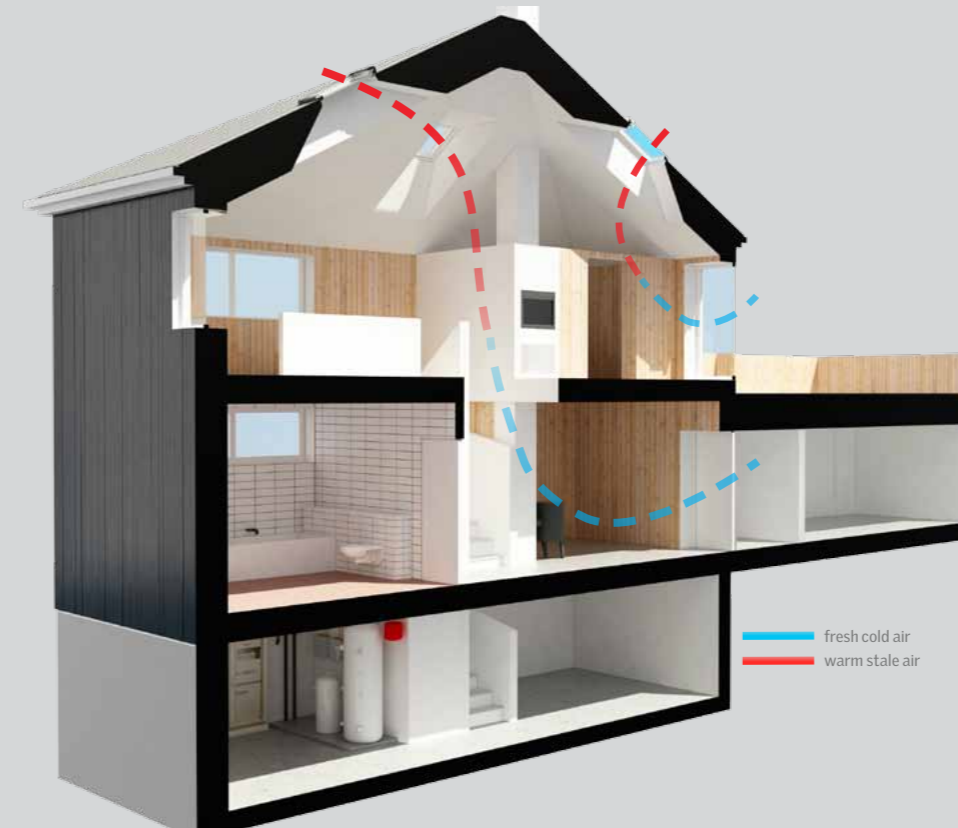
During summer natural ventilation ensures that the house is cooled and fresh air supplied in a way that significantly reduces the demand for electric fans. Furthermore, openable windows are appreciated by most users in the warm part of the year.
